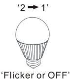
3. If load flickers or turns OFF, with the remote control press 'ON' button once to adjust one level higher ' $1 \rightarrow 2$ '
