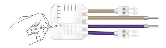
2. With a remote control press the '**ON**' button; LED on module will flash to confirm that the remote control is now paired.
