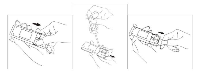
Replace with a new battery then slide up the battery cover.
