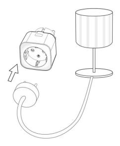
2. Plug the socket switch into an electrical outlet.
