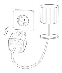
3. Within 6 seconds, on the remote control press the '**ON**' button intend to be paired; LED on socket switch will quick flash and load will flash twice to confirm that the remote control is now paired.
