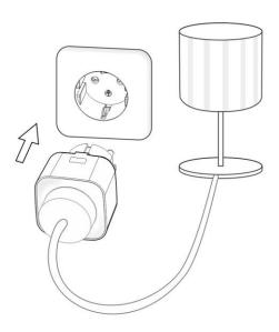
3. Within 6 seconds, on the remote control press the '**OFF**' button intend to be un-paired; LED on socket switch will quick flash and load will flash twice to confirm that the remote control is un-paired.
