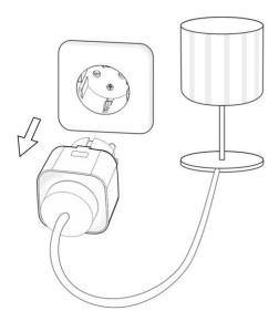
2. Plug socket switch back into electrical outlet.
