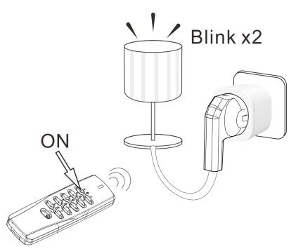
**NOTE:** If no signal is received from a remote control within 6 seconds then the socket switch will automatically exit learning mode without pairing the device.
