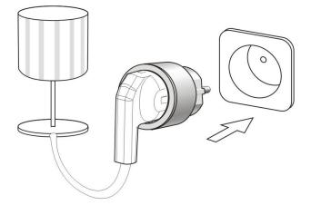
3. Within 6 seconds, on the remote control press the 'ALL OFF / GROUP ALL' button; load will flash twice to confirm all memory stored inside the socket switch has been deleted.
