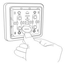
3. Replace with a new battery then place back the rocker cabinet.
