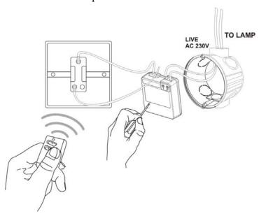
**NOTE:** Learning mode lasts for 12 seconds; if no signal is received from a remote control during this time then the module will automatically exit learning mode without pairing the device.
