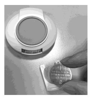
5. Slide back battery compartment to complete the battery installation
