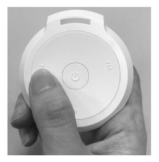
Turn the load ON: Press channel I button once. Red LED quick flash once.
