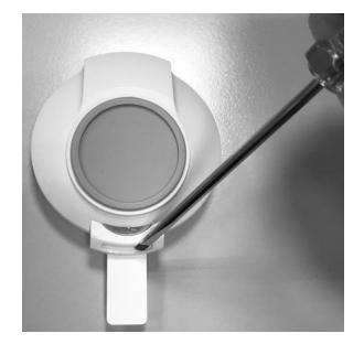
1. With a slot screwdriver carefully slide down the battery compartment.
