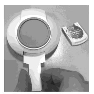
4. Remove 3V CR2032 battery and replace a new one making the positive symbol is facing upwards.
