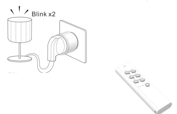
**NOTE:** If no signal is received from a remote control within 6 seconds then the socket switch will automatically exit learning mode without pairing the device.
