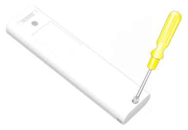
2. With a little force squeeze both side and pull out the battery compartment and remove 3V CR2032 battery.
